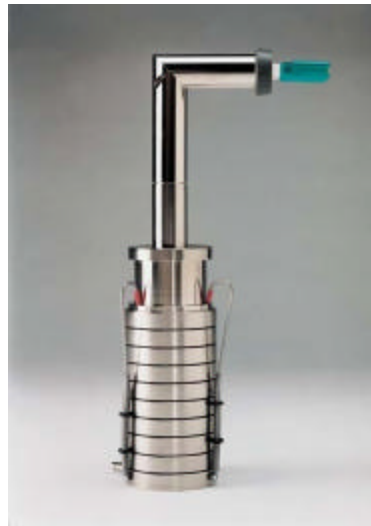
Figure 2: Andersen-Style Cascade Impactor with USP Pre-separator and Throat
